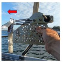
Assemble the line steerer with two 16 mm long bolts, washers and nuts, so that it points in the direction that the line is pulled out.
