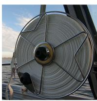
Adjust the brake knob, so that the line runs out smoothly. Attach preferable mooring hook, and your reel is ready for use.
