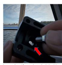
Insert the 12 mm long bolt inside the flat connector half before mounting it on the rail.
