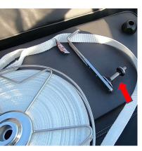
Relese the brake knob and take off the spool. **Note** how the washers are placed, to make sure how to re-assembly them.
